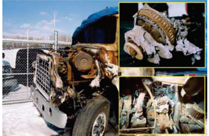
An alternator failure resulted in the engine fire of this truck. The insets show the destroyed engine compartment and alternator.
