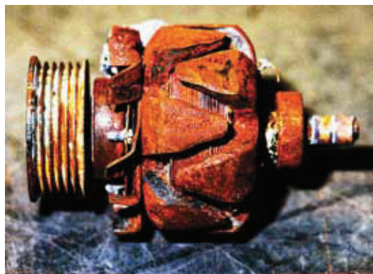
This rotor from a fire-damaged Lundell alternator shows the unique "claw-pole" configuration.
