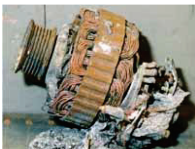
The above alternator, the cause of the engine fire pictured on the right, had actually fallen from its original mounted position on the front of the engine. It was recovered by the fire department.
