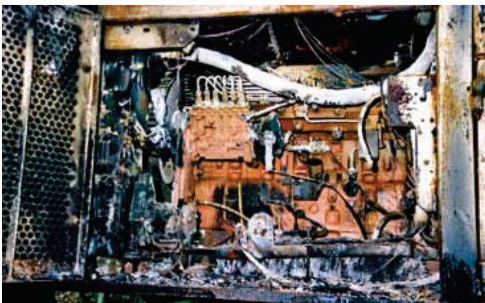
An alternator caused fire in a parked logging machine burned itself out over the night and was discovered the next day.
