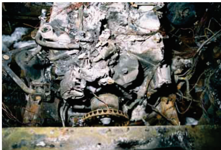
An alternator caused fire in a parked logging machine burned itself out over the night and was discovered the next day.
