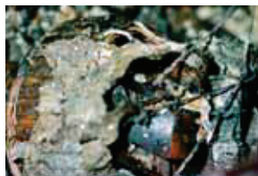
An engine compartment fire NOT caused by alternator failure. Note the lack of damage to the alternator.
