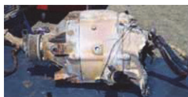
The damaged alternator after it was removed from the bus engine.
