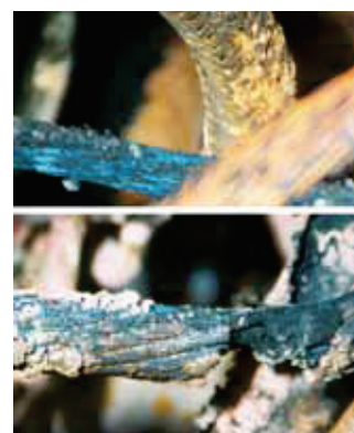
Two views of the cable between the battery and the alternator which was the source of ignition.
